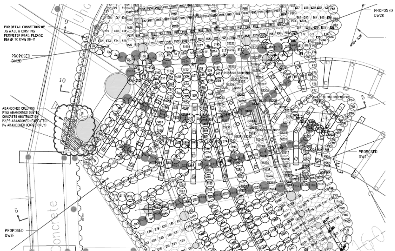
Figure 4: Complex layout of JG columns under SWSOOS
